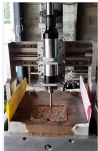
Figure 4.4 Processes Running a CAM Program with G code MDF wood material.
